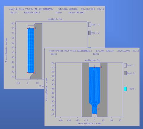
Design of a cold forming process
