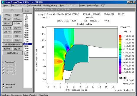
Failure of a punch
