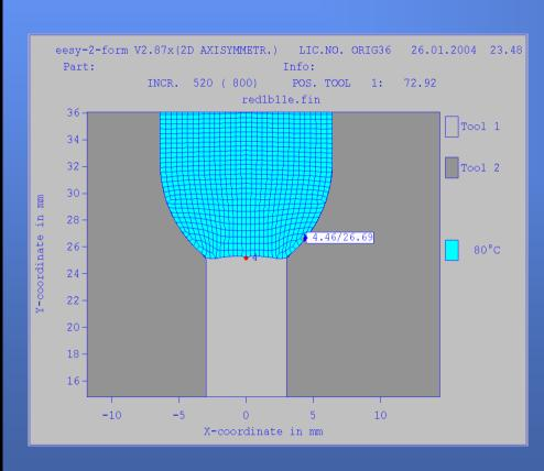
Design of a cold forming process
