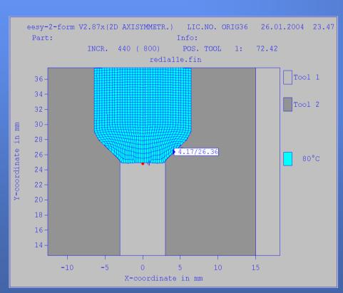
Design of a cold forming process
