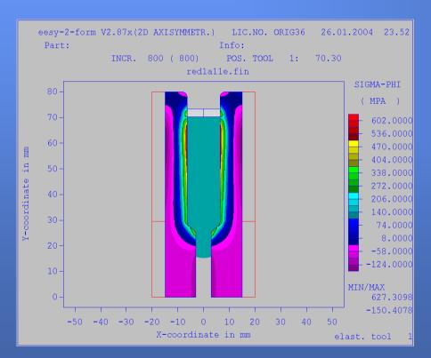
Design of a cold forming process
